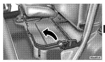
**Unfolding The Load Floor**
